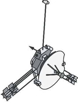
Satellites are also used for observation and research. A satellite can be placed in a **geosynchronous** orbit, which means that it can watch one particular location (such as Edmonton, Alberta) 24 hours a day. The satellite spins at the same rate as Earth. This type of satellite is useful for predicting and tracking the weather. Other satellites that are not in a geosynchronous orbit can observe forest fires, monitor soil quality, scout natural resources, and even follow ships at sea.
